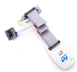
firmware is meant to only be used with radiometric FLIR Leptons (Currently the FLIR Lepton 2.5). Y16 firmware allows for the temperature to be read from each pixel on the Lepton, but it requires the use of specialized software to display such as our open source <a href="Mailto:GetThermal">GetThermal</a> application for MacOS and Linux.
